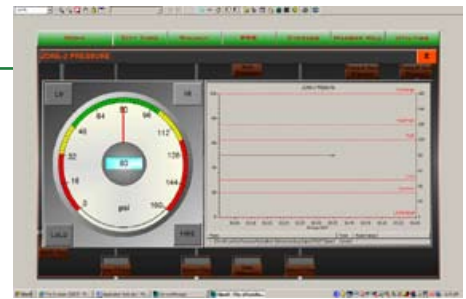
Figure #2, Zone 2 Pressure trending & alarming.
